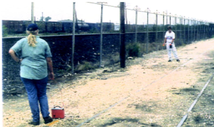
Radio-frequency utility line location at a Texas military base.
